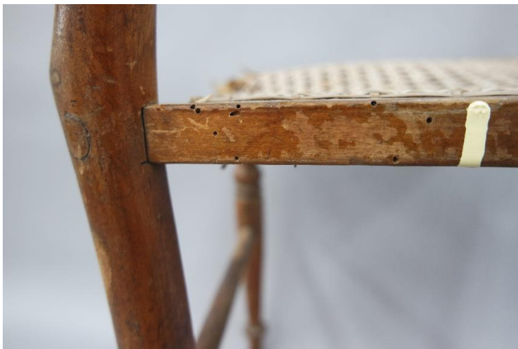
Fig. 15 Detail view on the seat frame from the back depicting, woodworm holes and paint drip.
